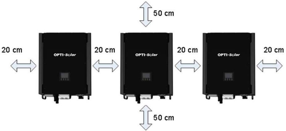
**NOTE:** For proper air circulation to dissipate heat, it's necessary to allow a clearance of approx. 20 cm to the side and approx. 50 cm above and below the unit. Be sure to install each unit in the same level.
